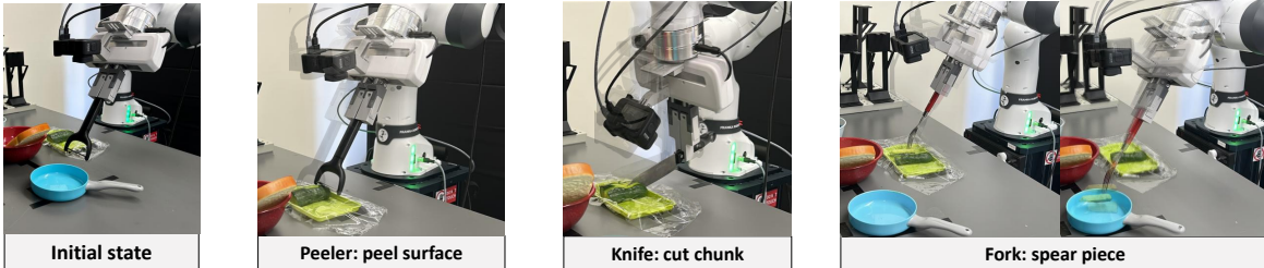
Fig. 5. We evaluate our system on two long-horizon tasks. Sandwich Assembly: the robot 1) picks and places bread, 2) scoops filling, 3) flips the fried egg onto the bread. Cucumber Preparation: the robot 1) uses the peeler to peel the cucumber, 2) cuts it in half with a knife, 3) uses a fork to spear the cucumber chunk into the pot.
